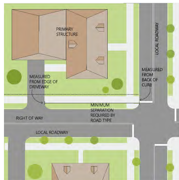
Example of Driveway/Intersection Separation
